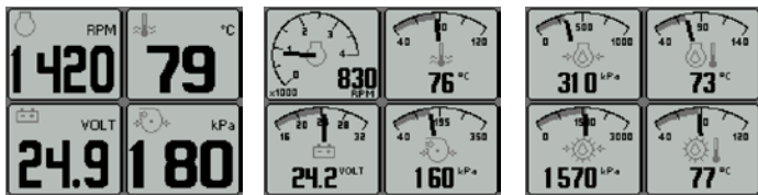
Figure 4. Top row: the 3 default displays available in quad-display, and adjust mode (right) which allows users to select the gauges displayed.
